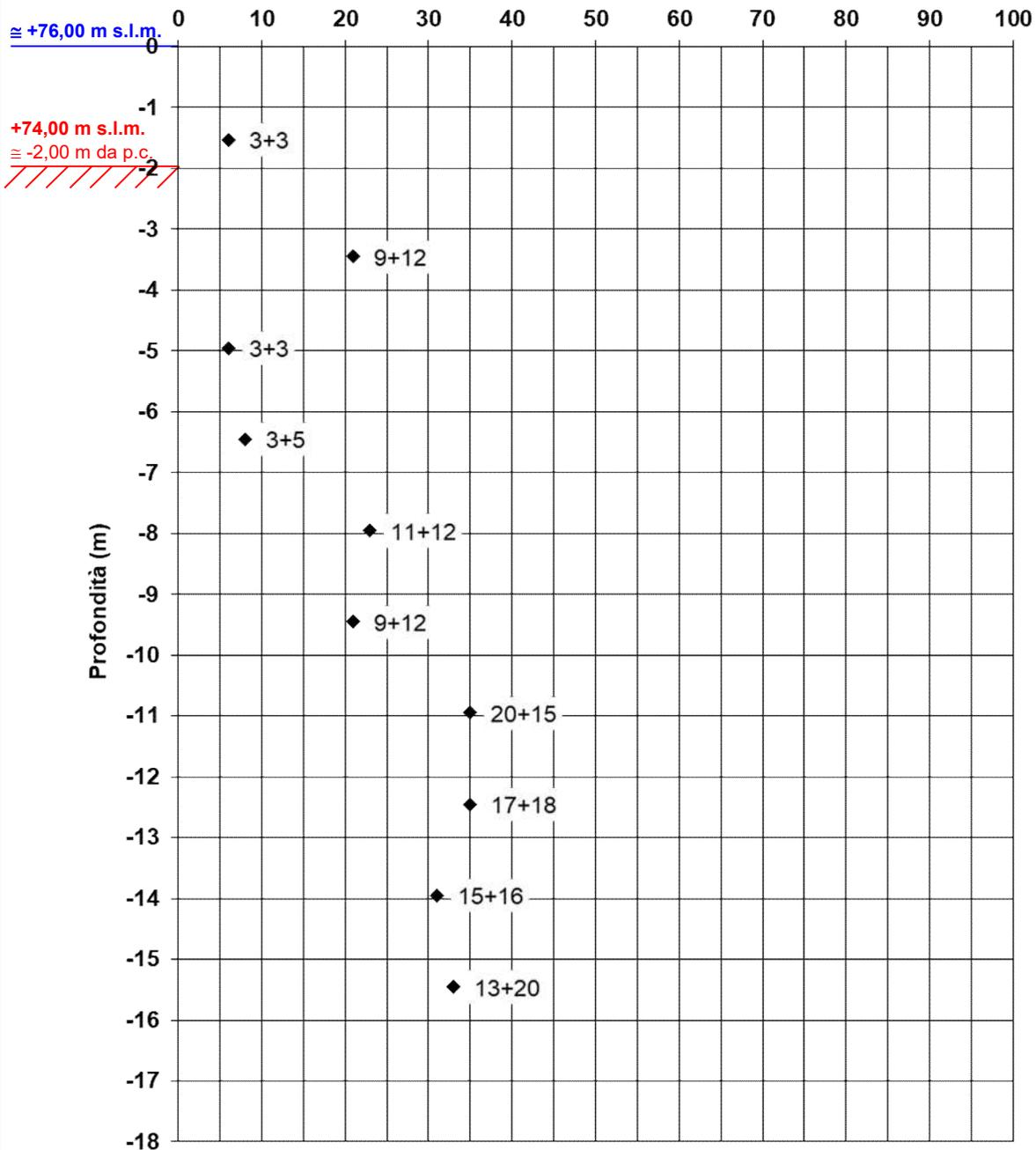
PROVE S.P.T. (STANDARD PENETRATION TEST) CON PUNTA CONICA: *Maglio 63.5 kg - Volata 76 cm*
